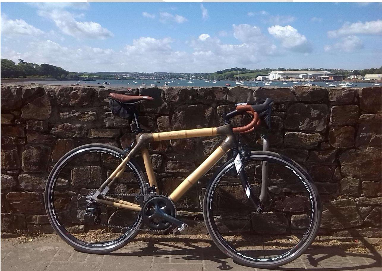
Figure 3 - Bamboo bicycle built by the author 5 years ago, incorporating hand-wound hemp fibre lugs – still in use.
