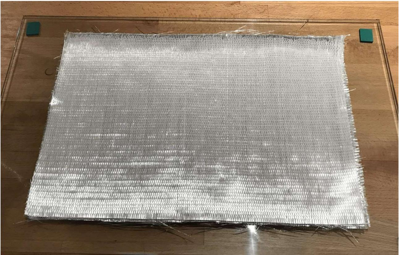
Figure 2 - Stack of E-glass plies, waiting to be infused at Orthotropic
